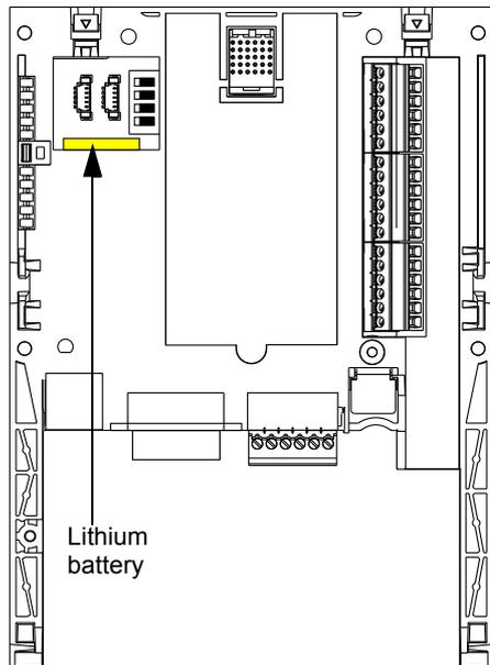
When installing the Water Solution card in the drive, make sure that this battery is present. It takes the form of a rectangular block clipped onto the non-volatile RAM (schematic opposite).
