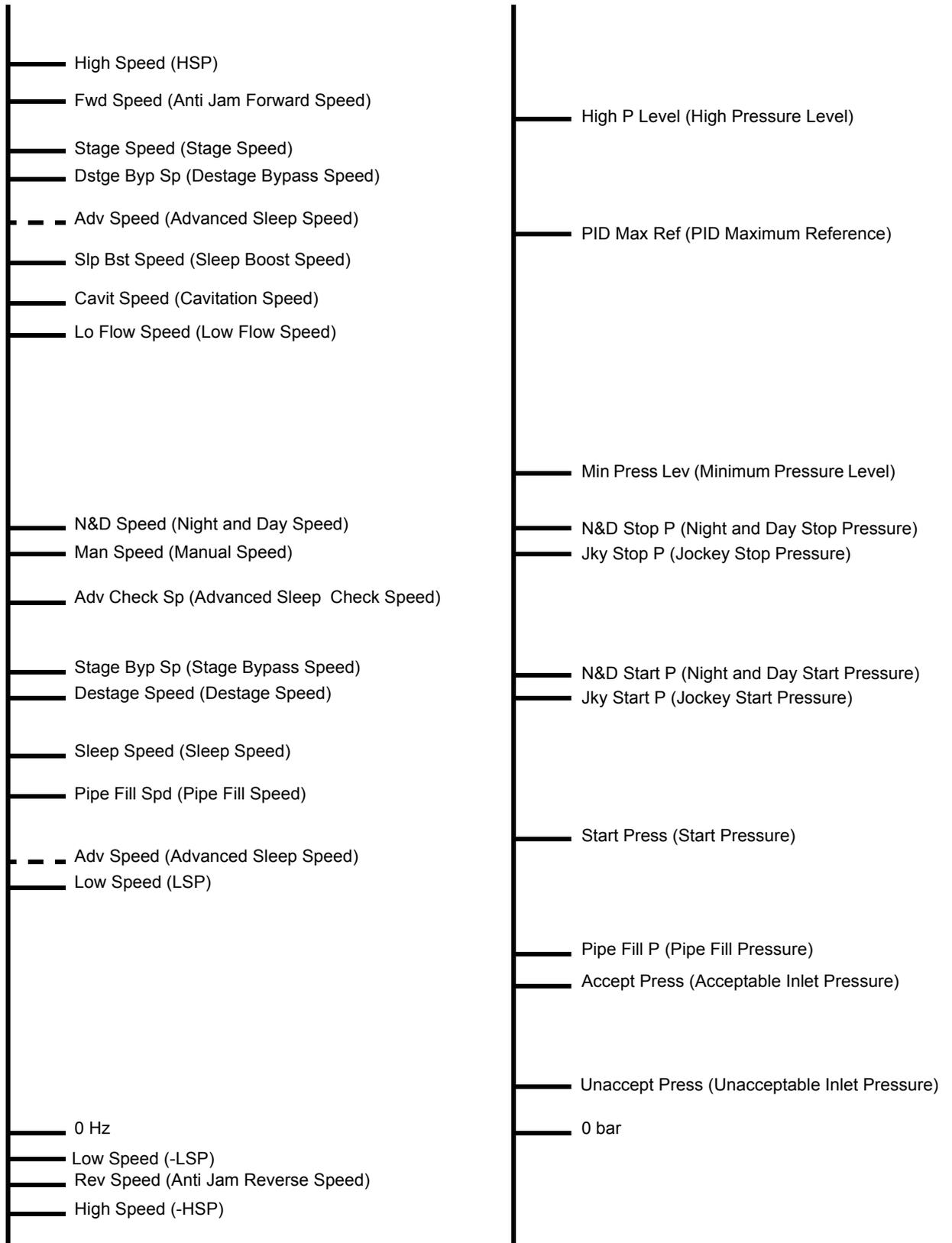
Note: The diagram above represents a scale of the recommended values for speed and pressure. For example, the recommended value for Fwd Speed (Anti Jam Forward Speed) is between High Speed (HSP) and Stage Speed (Stage Speed).
